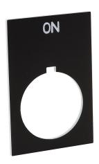
AutomationDirect legend plate, plastic, rectangular, black field, black background, white engraved text, legend plate marking "ON". For use with 22mm pilot devices. O-ring included.
