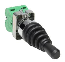
AutomationDirect selector switch, IP65, 22mm, 2-position, maintained, (2) N.O. contact(s), metal base, metal bezel, Operator: black, joystick, 30mm, round, plastic.
