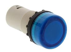
AutomationDirect incandescent indicating light, permanent light function, IP65, 22mm, blue, 30mm, round, plastic base, 24 VAC/VDC, full voltage.
