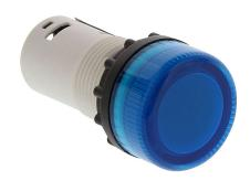
AutomationDirect incandescent indicating light, permanent light function, IP65, 22mm, blue, 30mm, round, plastic base, 120 VAC/VDC, full voltage.
