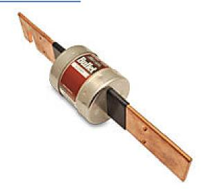
Edison fuse, ECSR series, Class RK5, current-limiting, time-delay, 450A, 600 VAC, knife blade, feeder/branch protection applications.
