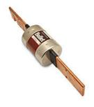
Edison fuse, ECSR series, Class RK5, current-limiting, time-delay, 250A, 600 VAC, knife blade, feeder/branch protection applications.
