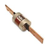
Edison fuse, ECSR series, Class RK5, current-limiting, time-delay, 225A, 600 VAC, knife blade, feeder/branch protection applications.
