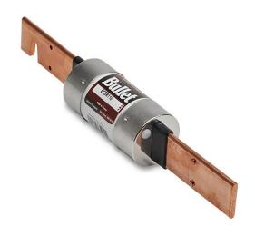
Edison fuse, ECSR series, Class RK5, current-limiting, time-delay, 110A, 600 VAC, knife blade, feeder/branch protection applications.
