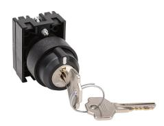
NITRA pneumatic selector switch, IP65, 22mm, 3-position, maintained, key removable in all positions, operator only, plastic base, plastic bezel, Operator: black, key, 30mm, round, plastic.
