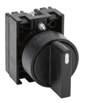
NITRA pneumatic selector switch, IP65, 22mm, 3-position, spring return to center from right or left, operator only, plastic base, plastic bezel, Operator: black, knob, 30mm, round, plastic.
