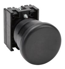
NITRA pneumatic pushbutton, IP65, 22mm, momentary, operator only, plastic base, plastic bezel, black, Operator: black, mushroom, 40mm, round, plastic.
