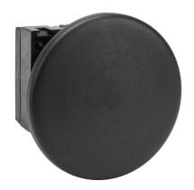
NITRA pneumatic pushbutton, IP65, 22mm, momentary, operator only, plastic base, plastic bezel, black, Operator: black, mushroom, 60mm, round, plastic.
