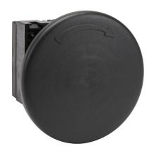
NITRA pneumatic pushbutton, IP65, 22mm, twist-to-release, operator only, plastic base, plastic bezel, black, Operator: black, mushroom, 60mm, round, plastic.
