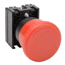
NITRA pneumatic emergency stop pushbutton, IP65, 22mm, twist-to-release, operator only, plastic base, plastic bezel, black, Operator: red, mushroom, 40mm, round, plastic.
