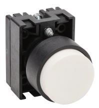
NITRA pneumatic pushbutton, IP65, 22mm, momentary, operator only, plastic base, plastic bezel, black, Operator: white, extended, 30mm, round, plastic.
