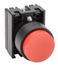
NITRA pneumatic pushbutton, IP65, 22mm, momentary, operator only, plastic base, plastic bezel, black, Operator: red, extended, 30mm, round, plastic.
