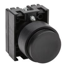
NITRA pneumatic pushbutton, IP65, 22mm, momentary, operator only, plastic base, plastic bezel, black, Operator: black, extended, 30mm, round, plastic.
