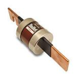
Edison fuse, ECNR series, Class RK5, current-limiting, time-delay, 500A, 250 VAC, knife blade, feeder/branch protection applications.
