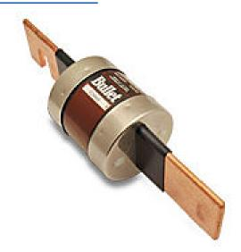
Edison fuse, ECNR series, Class RK5, current-limiting, time-delay, 450A, 250 VAC, knife blade, feeder/branch protection applications.
