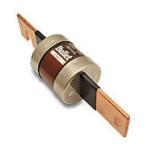
Edison fuse, ECNR series, Class RK5, current-limiting, time-delay, 450A, 250 VAC, knife blade, feeder/branch protection applications.
