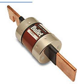
Edison fuse, ECNR series, Class RK5, current-limiting, time-delay, 350A, 250 VAC, knife blade, feeder/branch protection applications.
