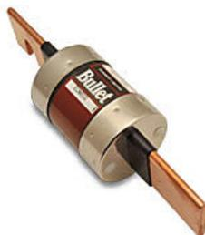
Edison fuse, ECNR series, Class RK5, current-limiting, time-delay, 300A, 250 VAC, knife blade, feeder/branch protection applications.
