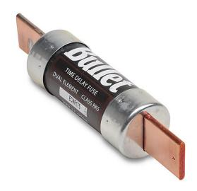
Edison fuse, ECNR series, Class RK5, current-limiting, time-delay, 175A, 250 VAC, knife blade, feeder/branch protection applications.
