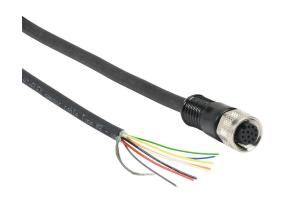
Lika Electronic encoder cable, M12 axial female to pigtail, shielded, 32.8ft/10m cable length. For use with Lika Electronic AQ58 and AQ59 series encoders.
