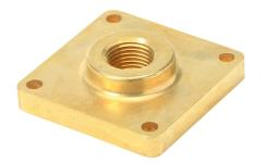
CITO port adapter, 1/2in female NPT, brass. For use with CITO StackFlow valves body inlet. BK-9100 inlet mounting kit included.
