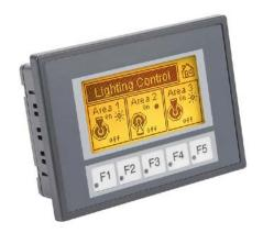
**C-more** Micro EA3 series HMI, 3in monochrome STN LCD, 128  $\times$  64 pixel, LED backlight, (1) serial port.
