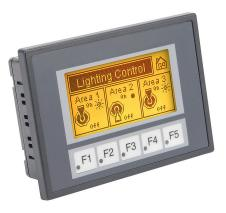
C-more Micro EA3 series HMI, 3in monochrome STN LCD, 128 x 64 pixel, LED backlight, (1) serial port.
