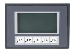
C-more Micro EA1 series HMI, 3in monochrome STN LCD, 128 x 64 pixel, LED backlight, (1) serial port.
