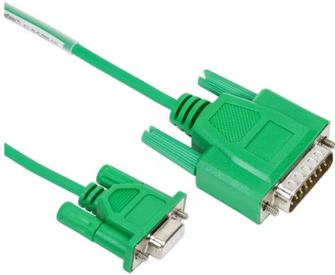
AutomationDirect communication cable, 15-pin male D-sub to 9-pin female D-sub, shielded, 3m/9.8ft cable length. For use with C-more or C-more Micro panel and an Allen-Bradley SLC 5/03, 5/04 or 5/05 CPU with DF-1 port.
