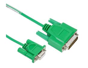
AutomationDirect communication cable, 15-pin male D-sub to 9-pin female D-sub, shielded, 3m/9.8ft cable length. For use with C-more or C-more Micro panel and an Allen-Bradley SLC 5/03, 5/04 or 5/05 CPU with DF-1 port.
