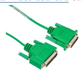
AutomationDirect communication cable, 15-pin male D-sub to 25-pin male D-sub, 3m/9.8ft cable length. For use with C-more or C-more Micro panel and an Allen-Bradley PLC-5 CPU with a DF1 port.
