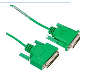
AutomationDirect communication cable, 15-pin male D-sub to 25-pin male D-sub, 3m/9.8ft cable length. For use with C-more or C-more Micro panel and an Allen-Bradley PLC-5 CPU with a DF1 port.
