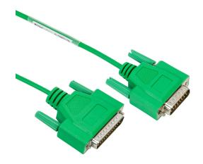
AutomationDirect communication cable, 15-pin male D-sub to 25-pin male D-sub, shielded, 3m/9.8ft cable length. For use with C-more or C-more Micro panel and an Omron C200 or C500 CPU.
