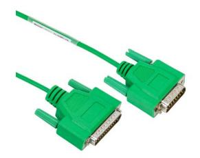
AutomationDirect communication cable, 15-pin male D-sub to 25-pin male D-sub, shielded, 3m/9.8ft cable length. For use with *C-more* or *C-more* Micro panel and an Omron C200 or C500 CPU.
