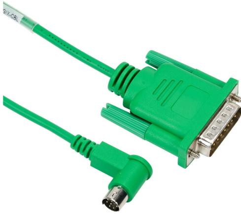
AutomationDirect communication cable, 15-pin male D-sub to 8-pin male mini DIN, shielded, 3m/9.8ft cable length. For use with C-more or C-more Micro panel and an Allen-Bradley Micrologix CPU.
