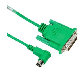
AutomationDirect communication cable, 15-pin male D-sub to 8-pin male mini DIN, shielded, 3m/9.8ft cable length. For use with C-more or C-more Micro panel and an Allen-Bradley Micrologix CPU.
