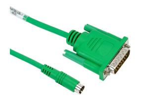
AutomationDirect communication cable, 15-pin male D-sub to 8-pin male mini DIN, shielded, 3m/9.8ft cable length. For use with C-more or C-more Micro panel and a Mitsubishi FX Series CPU.
