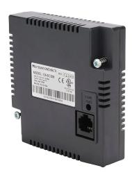
C-more communication expansion module, (1) RJ45 10/100 Mbps Ethernet port. For use with C-more Micro EA3 series 6in, 8in and 10in panels and all C-more HMIs except CM5 series and -R models.
