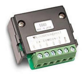
C-more DSUB port adapter, 15-pin male to 6-pole RS-422/485 terminal block, right angle cable entry. For use with C-more Micro EA1 series 4in and 6in HMIs, C-more Micro EA3 series 3in, 4in, and 6in HMIs, C-more EA9 6in and 7in HMIs and C-more CM5 series 4in HMI.
