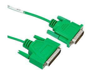
AutomationDirect communication cable, 15-pin male D-sub to 25-pin male D-sub, shielded, 3m/9.8ft cable length. For use with C-more or C-more Micro panel and a D2-DCM, D3-232-DCU, D3-350 (bottom port) or DL405 (bottom port) CPU.
