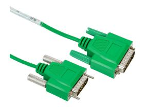
AutomationDirect communication cable, 15-pin male D-sub to 15-pin male D-sub, shielded, 3m/9.8ft cable length. For use with C-more or C-more Micro panel and a DL405 (top port) CPU.
