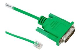
AutomationDirect communication cable, 15-pin male D-sub to 4-pin RJ11, shielded, 3m/9.8ft cable length. For use with C-more or C-more Micro panel and a D3-340 CPU top or bottom port.
