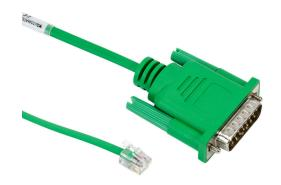
AutomationDirect communication cable, 15-pin male D-sub to 4-pin RJ11, shielded, 3m/9.8ft cable length. For use with C-more or C-more Micro panel and a D3-340 CPU top or bottom port.
