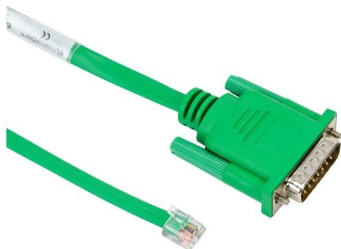
AutomationDirect communication cable, 15-pin male D-sub to 6-pin RJ12, shielded, 9.8ft/3m cable length. For use with C-more or C-more Micro panel and AutomationDirect PLCs with RJ12 ports.
