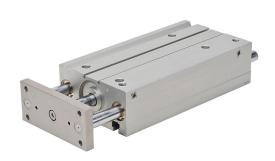
NITRA pneumatic cylinder, dual guide rod, 63mm bore, 20mm rod diameter, 250mm stroke, double acting, magnetic piston, universal mount.
