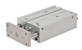
NITRA pneumatic cylinder, dual guide rod, 63mm bore, 20mm rod diameter, 200mm stroke, double acting, magnetic piston, universal mount.
