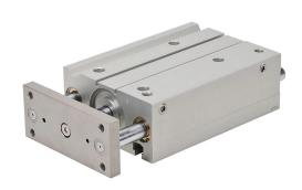
NITRA pneumatic cylinder, dual guide rod, 63mm bore, 20mm rod diameter, 175mm stroke, double acting, magnetic piston, universal mount.
