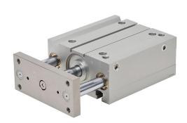
NITRA pneumatic cylinder, dual guide rod, 63mm bore, 20mm rod diameter, 125mm stroke, double acting, magnetic piston, universal mount.
