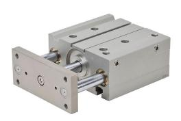
NITRA pneumatic cylinder, dual guide rod, 63mm bore, 20mm rod diameter, 100mm stroke, double acting, magnetic piston, universal mount.
