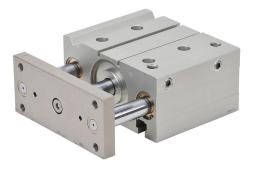
NITRA pneumatic cylinder, dual guide rod, 63mm bore, 20mm rod diameter, 75mm stroke, double acting, magnetic piston, universal mount.
