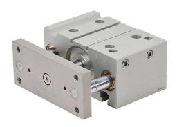
NITRA pneumatic cylinder, dual guide rod, 63mm bore, 20mm rod diameter, 50mm stroke, double acting, magnetic piston, universal mount.
