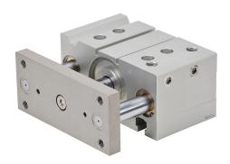
NITRA pneumatic cylinder, dual guide rod, 63mm bore, 20mm rod diameter, 40mm stroke, double acting, magnetic piston, universal mount.
