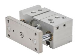
NITRA pneumatic cylinder, dual guide rod, 63mm bore, 20mm rod diameter, 30mm stroke, double acting, magnetic piston, universal mount.
