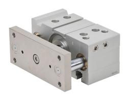
NITRA pneumatic cylinder, dual guide rod, 63mm bore, 20mm rod diameter, 25mm stroke, double acting, magnetic piston, universal mount.
