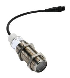
Eaton photoelectric sensor, tubular, threaded, 303 stainless steel housing, through-beam emitter, visible red light emission, 250m sensing distance, 10-30 VDC operating voltage, 2-wire, 4-pin M12 quick-disconnect.
