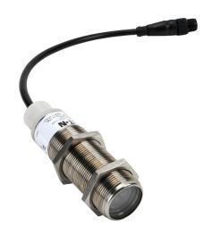
Eaton photoelectric sensor, tubular, threaded, 303 stainless steel housing, through-beam emitter, visible red, 250m sensing distance, 10-30 VDC operating voltage, 2-wire, 4-pin M12 quick-disconnect.
