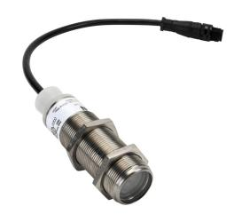
Eaton photoelectric sensor, tubular, threaded, 303 stainless steel housing, through-beam emitter, visible red light emission, 250m sensing distance, 15-30 VDC/20-132 VAC operating voltage, 2-wire, 4-pin AC micro 1/2in-20 UNF thread.
