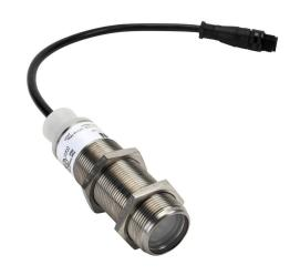
Eaton photoelectric sensor, tubular, threaded, 303 stainless steel housing, through-beam emitter, visible red, 250m sensing distance, 15-30 VDC/20-132 VAC operating voltage, 2-wire, 4-pin AC micro 1/2in-20 UNF thread.
