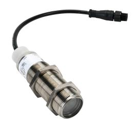
Eaton photoelectric sensor, tubular, threaded, 303 stainless steel housing, through-beam receiver, 250m sensing distance, 10-30 VDC operating voltage, light-on, NPN/PNP, 4-wire, 4-pin M12 quick-disconnect.
