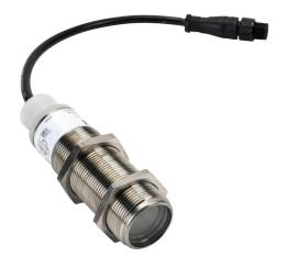
Eaton photoelectric sensor, tubular, threaded, 303 stainless steel housing, through-beam receiver, 250m sensing distance, 10-30 VDC operating voltage, light-on, NPN/PNP, 4-wire, 4-pin M12 quick-disconnect.
